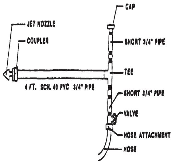
Water coming through the garden hose into the pipe is under pressure which will hydraulically drill a hole in the ground. The objective is to break through any impermeable soil conditions with the auger or water jet and allow water to drain away and air (oxygen) to enter the soil, improving the soil environment for growing roots.
