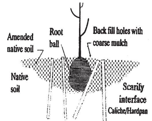
**Figure 1. Vertical mulching around and under trees and shrubs.**
