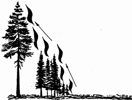
Figure 1. Smaller trees form a ladder-like configuration that contributes to fire spread into the crowns of larger trees. Removal of the smaller trees is similar to reducing rungs in a ladder—it makes it harder for fires to climb the fuel ladder.
