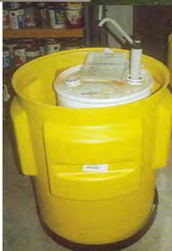
Left: Use a barrel or tub to contain pesticides stored on the floor or ground.
