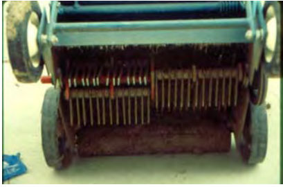
Fig. 4. Underside of a power rake, showing the blades.
